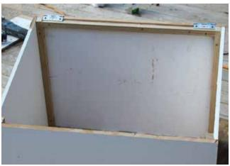
Fastening the lid to the chest with hinges can be done a number of ways and will depend on what type/style you have chosen. The easiest option is to fix 'butt' (as shown) or gate hinge leafs to outside faces of lid and back panels. If you prefer a concealed hinge, some rebating is required.
