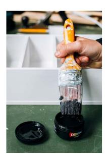
**4** Fill the screw holes with Resene EzyFill Quick and allow to dry. Sandpaper the box, then paint with Resene Quick Dry waterborne primer undercoat. Allow to dry completely, then follow with an overcoat, I used Resene Charcoal.
