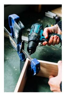
**1** To make the frame, fix together the side pieces and the top and bottom piece of pine clear to form a rectangle. Pre-drill all the screw holes with a 2mm drill bit, and then attach together using screws.
