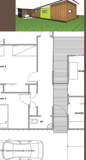
Aotearoa Housing is a student design proposal for an affordable housing option. It is aimed towards providing a higher quality and standard of living for Maori. It is envisaged that this will be built in transportable units that can be built and then transported or shipped to the site.
