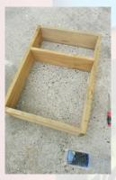
**Step five** Fit the first of the shelves, as shown, fixing through each side with 50mm screws.
