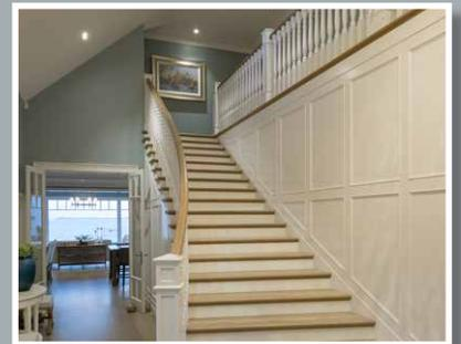
Painted in Environmental Choice approved **Resene Zylone Sheen** low sheen, with **Resene Enamacryl** gloss waterborne enamel on trims. The exterior is finished in **Resene Lumbersider** low sheen for its easy application and performance.
