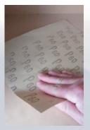
Step one Lightly sand the MDF cabinet to provide a 'key'.
