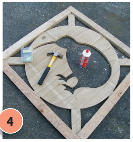
4 Glue with PVA glue and nail (with galvanised nails) four lengths of treated timber around the panel's front edges, as shown. Turn the panel over and attach the four remaining lengths around the back. Allow the glue to dry.
