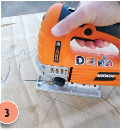
3 Rule a 'frame' around all the panel, 70mm in from its edges. Mark lines 35mm out on each side of the vertical, horizontal and diagonal lines (for 70mm inner 'supports'). Cut out the inner kiwi outline and outer triangular sections with a jigsaw.
