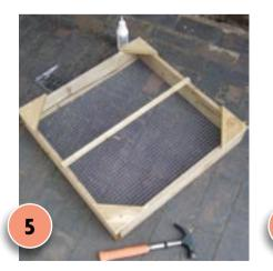
Measure and cut six small triangles of wood and attach to the base of the larger frame with PVA glue and nails. Measure and cut a 20mm reinforcing strip, and attach in the same way across the base.
