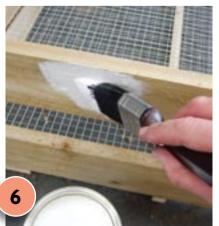
Apply one coat of Resene Quick Dry waterborne primer undercoat to all wooden parts of each frame. Allow to dry for two hours.
