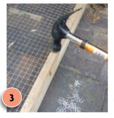
(a) Measure and cut a square of wire mesh to fit the larger frame and attach with galvanised staples, as shown.(b) Turn the outer frame upside down and place the smaller frame inside it.
