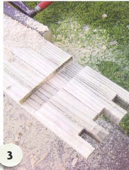
3 Turn the legs, as shown, and reclamp. Repeat step 2 to make two 50mm grooves across the legs, each one approx 150mm from either end.
