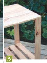
Make the top by drilling and screwing 7 of the 1m planks into place. Then add another 1m plank to the front (this is the board we painted pink).
