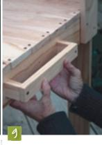
Finally, add the handles. Our handles are made from 25cm lengths of 4"x1" timber attached to a 4cm x 4cm block at each end.
