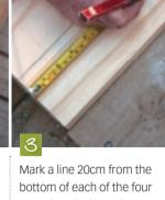
Mark a line 20cm from the bottom of each of the four 90cm leg planks and use these as a guide to screw the lower shelf to the legs.
