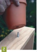
Drill three holes through the top of the back shelf and thread a bolt through the wood, into the terracotta pot. Secure with a nut and washer.
