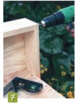
Build the back shelf by screwing the 32cm planks to each side of the table, then screwing the final three 1m planks to the side pieces.
