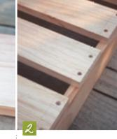
Build the bottom shelf first, using two of the 1m planks and eight of the 60cm planks.
