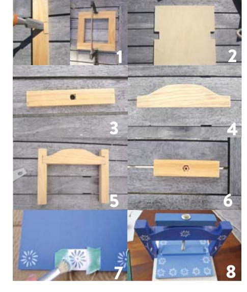
Cut out all the pieces. Mark a 30mm wide x 10mm deep cut-out in the centre of one side of the two long pieces. Using a hand saw or jigsaw, cut the two 1cm cuts. Use the chisel to create the cut-out and sand it smooth. Glue and clamp the base together and allow to dry. Drill a small guide hole through the centre of the cut-out.
