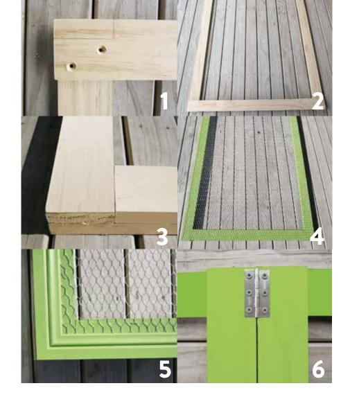
Mark screw holes into the top and bottom panels, making an allowance for the hinges to the top two panels.
