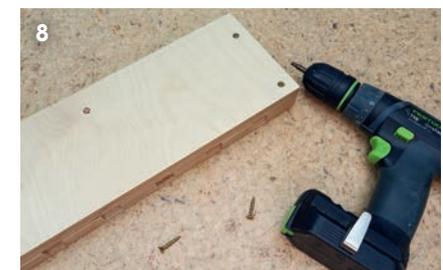
on the space pieces and drill 6 pieces all the way through, with 2 pieces only drilled half way for each end.
