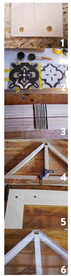
Base: Mark two screw holes 25mm in from the end on the longer lengths. Drill 5mm deep holes with the 18mm paddle bit. Drill a centre hole through the timber. Mark and drill the screw holes to match on the side pieces. Undercoat with Resene Quick Dry Primer. Topcoat in Lumbersider – I used White.
