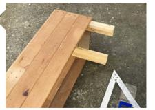
Step Six Measure, mark and cut six 300mm lengths from the recycled plywood strip. Then, measure, mark and cut two 730mm lengths from the remaining 45mm x 20mm recycled timber.
