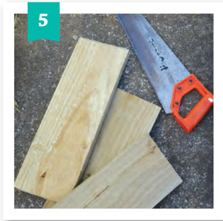
Use pencil lines as a guide to cut the fence paling into sections, as shown.
