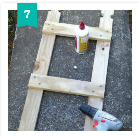
Use 40mm screws and PVA to attach the three 350mm lengths to the two 900mm picket fence palings, as shown. Use a set square to ensure that they are fixed at right angles and drill pilot holes first to prevent the wood from splitting.
