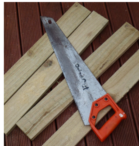
7. Cut the remaining two pieces of fence paling in half lengthways. Measure, mark and cut two of these lengths to 460mm, leaving the other two at 600mm. Smooth any rough edges with sandpaper.
