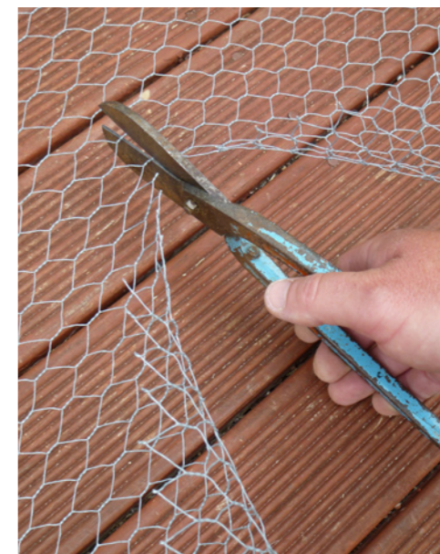
11. Cut pieces of chicken wire to fit the door frame and line the inside of the composter.
