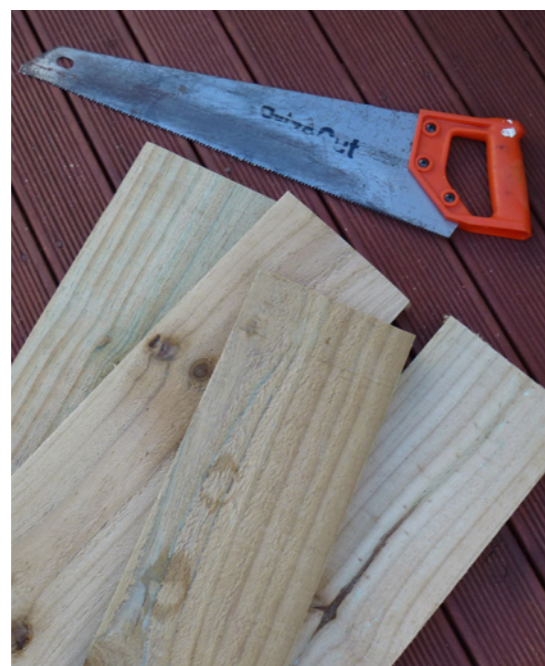
2. Cut the fence palings into 600mm lengths and cut the 50mm x 50mm timber into four lengths, each measuring 1.1m. Smooth any rough edges with sandpaper.
