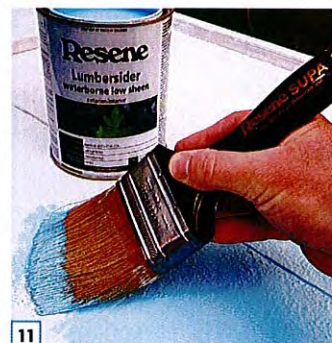
11 Paint the outside panels of the planter with two coats of Resene Anakiwa, allowing two hours for each coat to dry.
