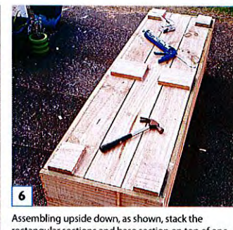
6 Assembling upside down, as shown, stack the rectangular sections and base section on top of one another. Run a line of construction glue between each section as you assemble the planter. Cut six small feet from the remaining pieces of fence paling and attach to the base with construction glue and 50mm nails.
