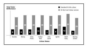
The full Cool Colour system is generally **Resene Cool Primer** plus two topcoats of Cool Colour topcoat, however with some colours the Resene Cool Primer only adds a minor improvement to the system so you can leave it out. Check with your Resene rep if you are planning to use a Cool Colour without the Cool Primer and they can confirm with Technical before you start to make sure the system will still work well.
