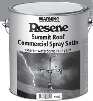
To spray, simply use an airless unit such as a Graco 395 capable of achieving a minimum flow rate of greater than 2 litres per minute and a 60 mesh manifold and gun filters. Spray set up is a FFCP 516 tip at 1400 psi.
