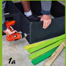
**Step 1:** Make the black frame by screwing the back and side panels together as shown, then attach the bottom plates of each box area. The long side panel goes in the middle and the short ones on the sides – one high and one low. Use stainless steel screws for longevity. Drill drainage holes in the base of the boxes.
