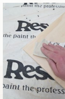
Step four Carefully sand the piece of plywood, running in the direction of the grain, smoothing any rough edges. Wipe off any sanding residue with a lightly damp sponge.
