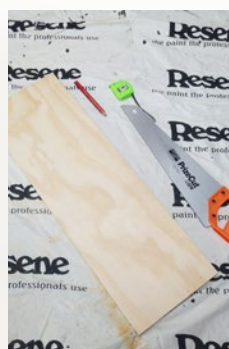
Step three Measure, mark and cut the piece of plywood to form a new top, ensuring a 10mm overhang along the side and front edges.
