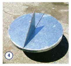
Glue the gnomon triangles together with construction adhesive, then cut a thin slot into the Zincalume circle (from the outer edge to centre). Glue the gnomon to the plywood circle, then glue the Zincalume circle into position, sliding the gnomon into the thin slot. Clamp until it dries. Glue the Zincalume band around the outer edge of the circle, fixing each end with a small panel pin.
