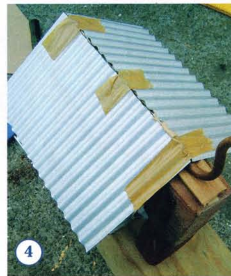
4 USING builders' construction adhesive, glue the front, side and roof zinalume panels to the mailbox, fixing in place with parcel tape until the glue has set. Screw the letterbox to an offcut of marine ply. Attach copper pipe to underside of roof with wire and glue.
