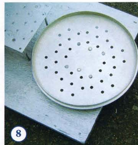
8 FINISH off with two coats of Resene Enamacryl in 'Silver Aluminium'. Allow to dry, then nail and glue the aluminium saucepan lid to form the feeding tray.
