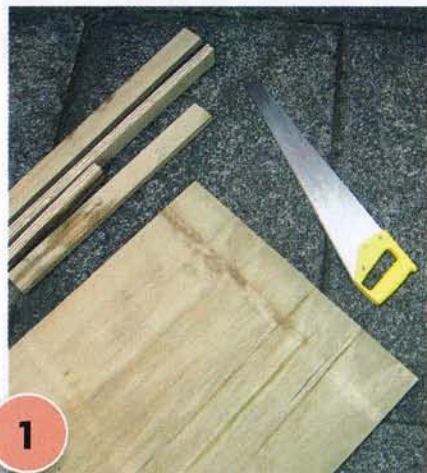
1 Measure, mark and cut the plywood to the dimensions listed above. Smooth any rough edges with sandpaper.
