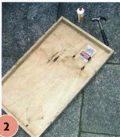
2 Assemble the art panel, as shown, fixing along each edge and at the corners with PVA glue and nails.
