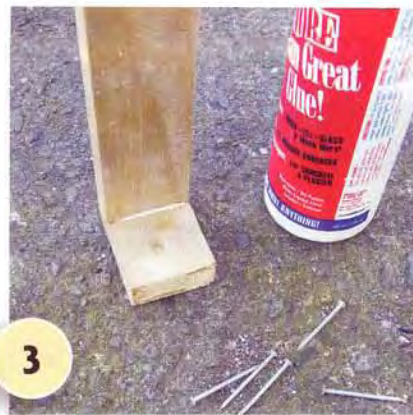
3 For the wall bracket, partly drill a 10mm hole in the centre of the smaller batten piece and then attach it to the base of the longer batten length, as shown. Fix with PVA glue and 40mm nails.
