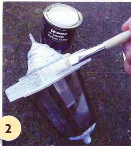
2 Apply one coat of Resene Smooth Surface Sealer to the top and base of the light.
