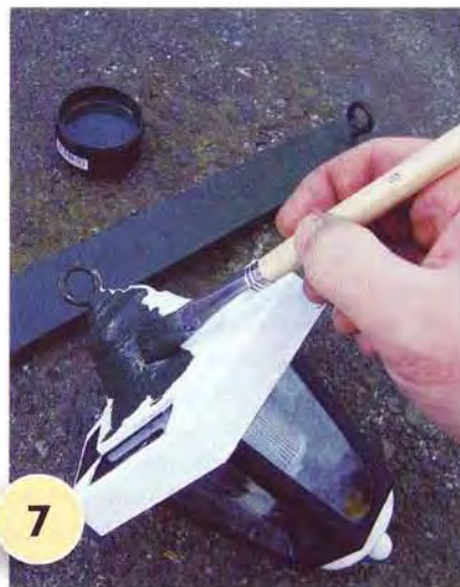
7 Apply two coats of Resene Midnight Moss to the base and top of the lamp and the wooden bracket and fix the bracket to a fence or wall with stainless steel screws. Drill pilot holes first.
