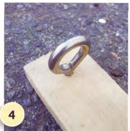
4 Attach the screw eye to the other end of the longer length of batten, drilling a pilot hole first. Lightly sand the screw eye to provide a key.
