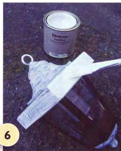
6 Apply one coat of Resene Mediterranean effect to the wooden bracket and also to the top and base of the lamp, as shown. Dab the paint on to create a textured effect. Allow to dry.
