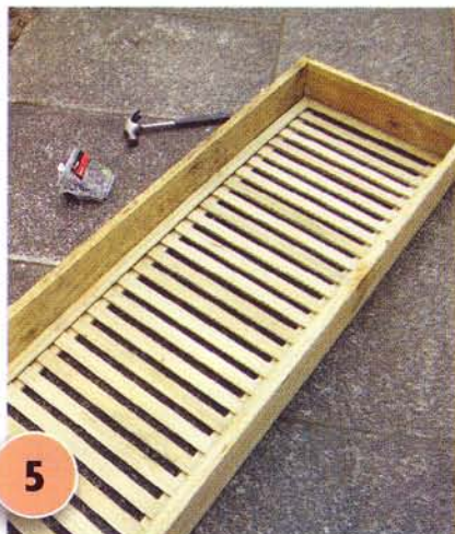
5 Make a 'frame' around the cut wooden panel, as shown, using two full 1.5m fence palings and two of the smaller cut lengths. Attach at each corner with galvanised nails and fix the wooden panel into position, by nailing through from the sides.
