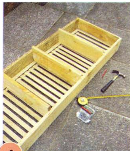
6 Fix the three shelves into position, as shown, nailing through from the sides.
