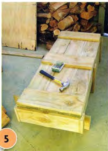
5 Turn upside down and fix the base into position using nails and glue, as shown.
