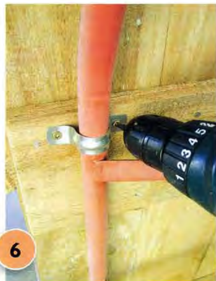
6 Attach the trolley to the underside of the planter, fixing the upright handles to the base with four galvanised 'half round' pipe brackets and 30mm screws.
