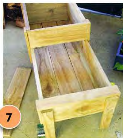
7 Turn planter right way up. Attach two legs at the front (as shown) – check their length as it will depend on the back wheel's size. Attach the last length of paling as a horizontal brace across the planter's front. Leave overnight for glue to dry.
